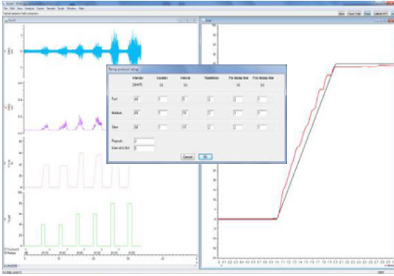
Force-time target following experiment. Script generated target template with overlaid subject response. Target recorded in data file with associated EMG
